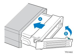
Figure 19. Inserting a Hot-swap Hard Disk Drive Assembly into the Chassis
